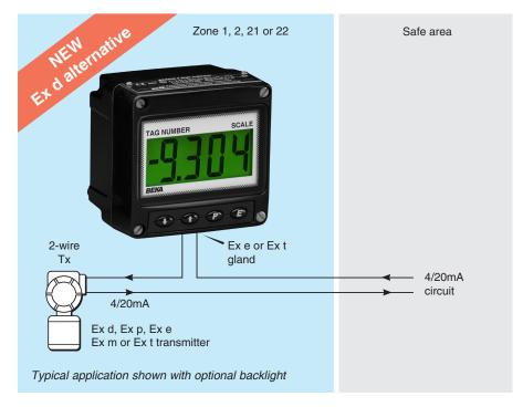
The BA304SG loop powered 4/20mA indicator is a new low cost alternative to a flameproof Ex d indicator featuring a large 34mm high display. Increased safety Ex eb and dust ignition protection by enclosure Ex to certification allow it to be safely installed in Zones 1, 2, 21 or 22 without the need for a Zener barrier or a galvanic isolator. Installation requirements are the same as those for an Ex d instrument.
