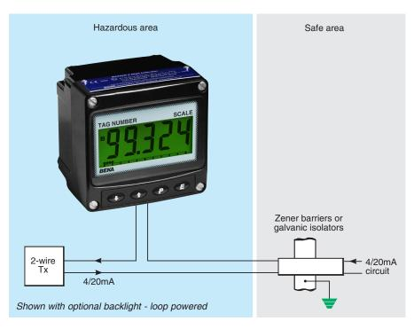
The BA324G loop powered 4/20mA indicator is a new field mounting instrument that supersedes the well established BA324C. It is electrically and mechanically compatible with the earlier model but has a much larger full 5 digit display and guaranteed performance between -40 and +70°C. Like it's predecessor, the BA324G is housed in a robust IP66 enclosure which may be surface or pipe mounting.
