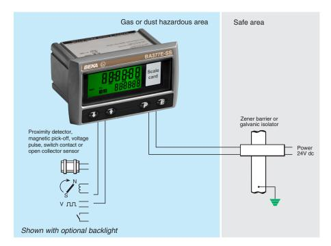
The BA377E-SS is an intrinsically safe instrument with one input housed in a rugged stainless steel enclosure that may be configured as a Timer or as a Clock. The intrinsic safety certification and the rugged enclosure allow the BA377E-SS to be safely installed in an Ex e, Ex n, Ex p or Ex t panel enclosure without invalidating the panel enclosure's certification.
