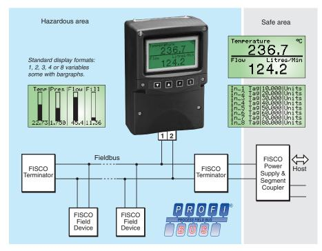
The BA484DF-P Fieldbus Display is an intrinsically safe instrument that can display up to eight fieldbus process variables. Eleven selectable standard screen formats contain one, two, three, four or eight variables, with units of measurement, tag descriptions and bargraphs on some screens.
