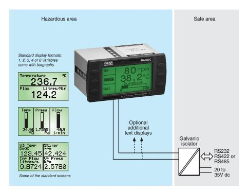
The BA488C is an intrinsically safe instrument that can display text and simple graphics in a hazardous area. Incorporating six push buttons and two solid state outputs, the BA488C is a low cost operator interface ideal for simple machine and process control applications. Incorporating Modbus RTU, BEKA and Legacy protocol the instrument may be used for new installations or to upgrade existing intrinsically safe systems.
