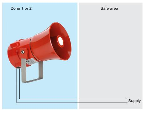
The BExS110D solid state electronic sounder produces a loud audible warning signal within a hazardous area. To avoid confusion between alarm signals, the sounder can be conditioned by internal switches to generate any one of thirty two unique alarm sounds. Maximum continuous output is 113dB(A) at 1m. **ATEX flameproof certification** allows all models to be installed in Zone 1 or 2, and to be used with gases in groups IIA, IIB and IIC.
