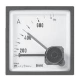
The thermal/time characteristics of MDI meters monitor the most economic use of cable, fusegear and transformers. The directly heated bimetal element indicates mean RMS current over 8, 15, or 20 minutes, and a red slave pointer shows the highest value reached. The reset knob is wire sealable. Scales are calibrated to match the CT primary plus 20% overload. End values are selected from: 1.2, 1.8, 2.4, 3, 3.6, 4.8, 6, 7.2, 9 amps and their multiples of 10 and 100.
