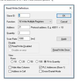
Define the register to write to. Below an example to change the network node id.
