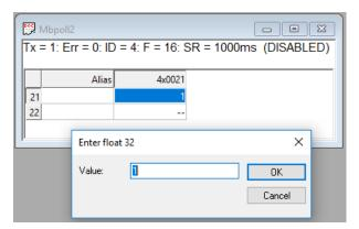
Press F8 and followed by a press on the Read/Write Once button to write the value to the meter
